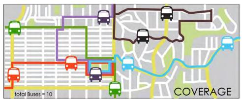
Figure 1: Schematic of coverage network model (fleet of 10 buses)
