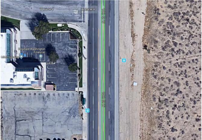
Figure 5: Example of an in-lane bus stops on 10<sup>th</sup> St W, but the northbound bus stop lacks a landing pad and safe pedestrian crossing.
